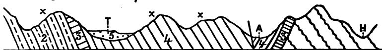
Section (4)—Mountains west of Tarndale, across Alma Valley to Acheron River. 1. Annelid beds. 2. Lower Trias. 3. Middle Trias (diabases with Monotis ). 4. Upper Trias, Lias, &c. 5. Recent or Pleistocene. T. Tarndale Flats. A. Alma River. H. Acheron River. x Fossil plants.
